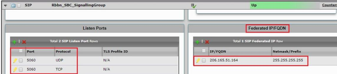
**IP Address/FQDN in Federated IP/FQDN:** Specifies the IP Address or Fully Qualified Domain Name of a server from which the SBC Edge 1000 accepts SIP messages. Make sure that it contains the IP address of the Asterisk PBX.
