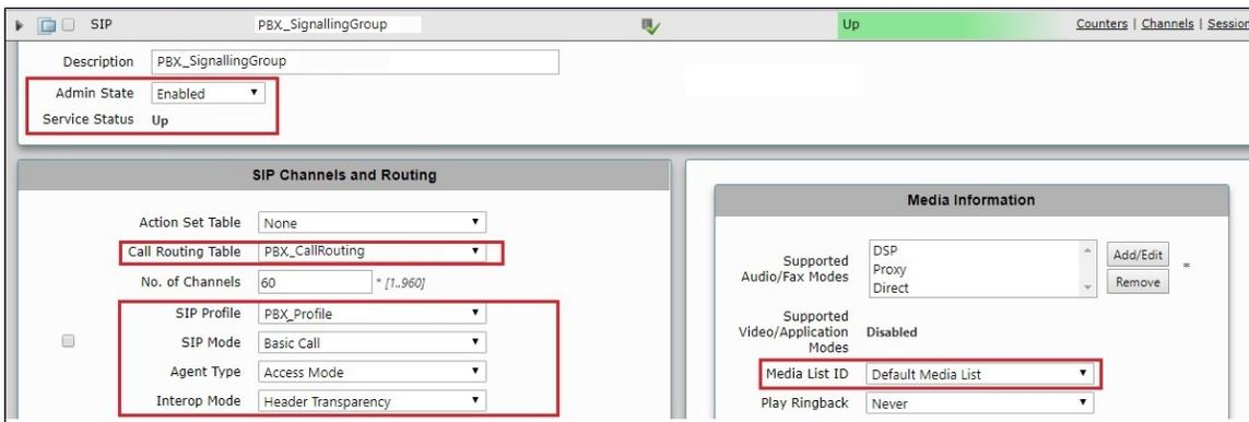
The image displays three screenshots of the PBX\_Profile\_SignallingGroup configuration interface, highlighting specific settings related to SIP configuration.
